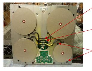
DISCONNECT WIRING FROM MAIN TERMINAL BLOCK
